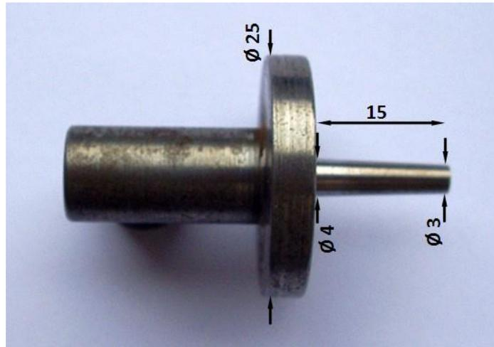
Figure 18: Test pin and dimensions
