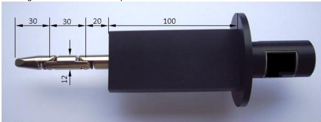
Figure 17: Test finger and dimensions
