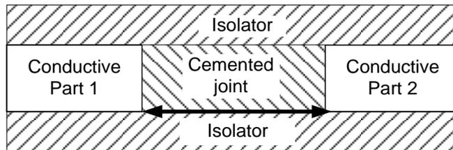
**Figure 4: Insulation on the same PCB layer require regular creepage and clearance distances**
