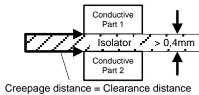
**Figure 3: Minimum thickness insulation material**
