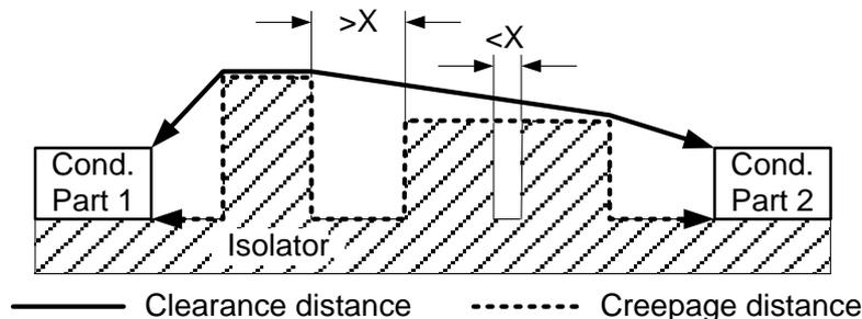
Figure 11: Determination of creepage and clearance distance
