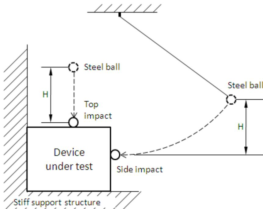
Figure 16: Steel ball test
