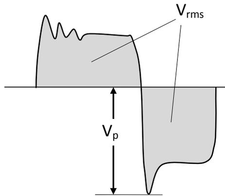
Figure 10: Example of working voltage measured between two points across an insulation
