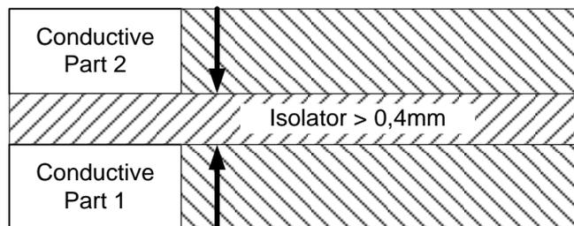
**Figure 5: Insulation between different PCB layers is reinforced, if distance is > 0,4mm or meet criteria in table 2R of the standards (e.g. min 3 layers of prepreg)**
