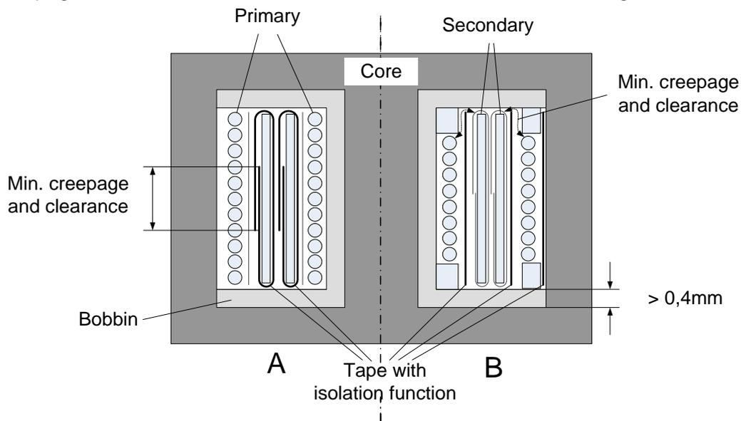
Figure 8: Cross section of an isolation transformer with double/reinforced insulation
