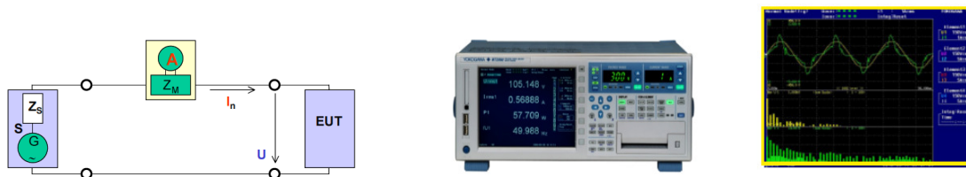
Figure 7. Harmonic current analysis
